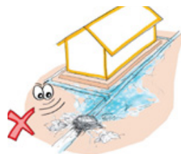
Having standing water in the surrounding area of the shelter that creates water logging
