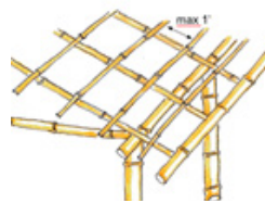
Distance between purlins is less than 1ft (30cm)
