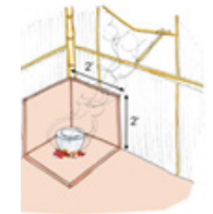
Having non-flammable materials protecting the walls in the cooking area
