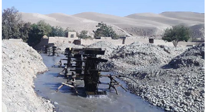
This community in Takhar has installed locally-made surface water pumps to carry water to farms from a stream through water pipes. © IOM 2021
