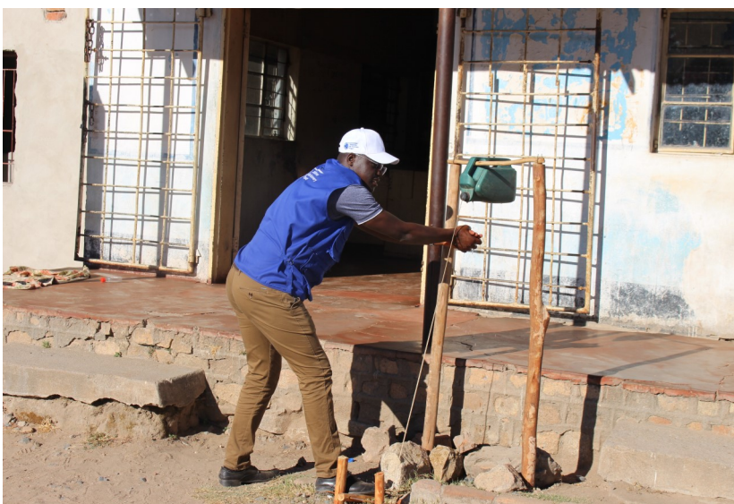
A makeshift foot-step hand washing station in front of a shop in Makoni. @IOM July 2020
